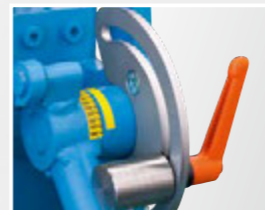
Adjust bending angle with scale and lever
