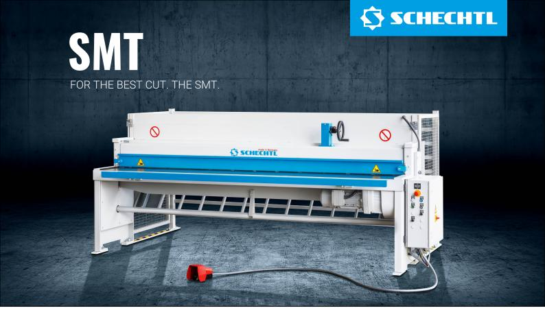
The Schechtl SMT is the entry-level model in our range of motorized plate shears. With its extensive range of equipment options, it offers a high degree of flexibility in the production process. With its compact design, it also offers maximum efficiency in the tightest of spaces. The cutting material tray can be perfectly adapted to suit the material flow in your workshop – simply select the tilting table version which deposits sheets towards the front or towards the rear ex works.
