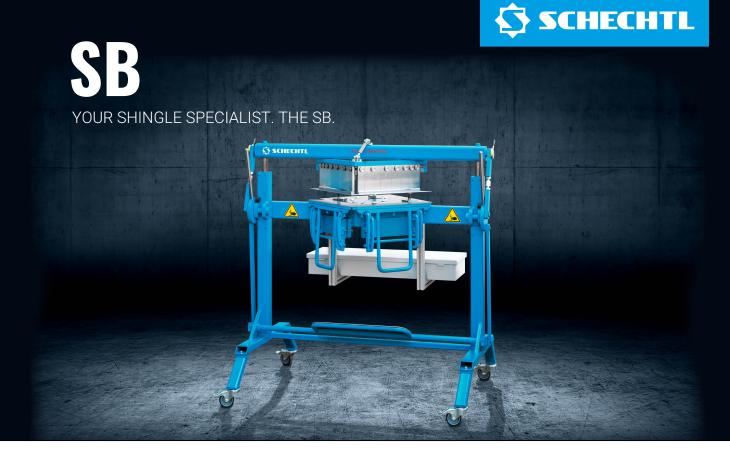
The Schechtl SB produces shingles quickly and simply. To do this, the SB bends two edges or hems which are arranged at an angle of 90 degrees to each other. The clamping beams are equipped with replaceable segments, making the production of square and rectangular shingles or other components extremely easy. In addition, with the SB, the usual 24 work steps are reduced to 8. This is a time-saving of approx. 70%.
