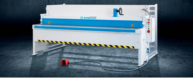
The Schechtl MSB is the reinforced version of the SMT. It is even more solidly constructed than the SMT, which means higher cutting performance. The cutting material tray can be perfectly adapted to suit the material flow in your workshop – simply select the tilting table version which deposits sheets towards the front or towards the rear ex works.
