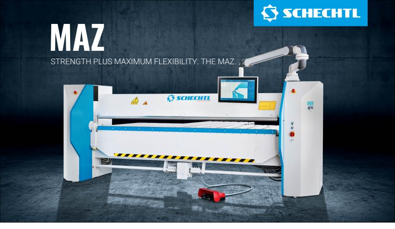
With cutting-edge technology, the Schechtl MAZ boosts productivity and flexibility in the production of metal edge profiles. The eccentric drive offers convincingly high clamping force. The Click System comes as standard, minimises set-up times and allows easy retrofitting of special tools at any time. At the same time, the solid, torsion-free welded construction ensures a long machine service life even with consistently heavy loads.
