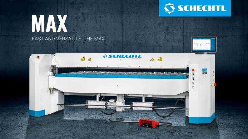
The Schechtl MAX is perfect where there is extensive work to be done on roofs and exteriors. With a range of control systems and backgauge options as well as a wide selection of rails, the MAX can be fully customised to suit your wishes.
