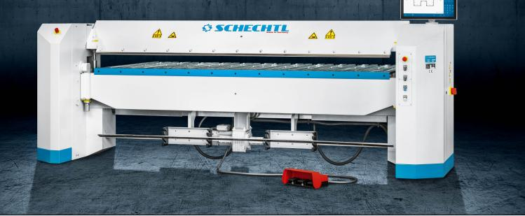
The Schechtl MAB is the reinforced version of the MAX. It is even more solidly constructed, which means greater bending capacity. With a range of control systems and backgauge options as well as a wide selection of rails, the MAB can be fully customised to suit your wishes.
