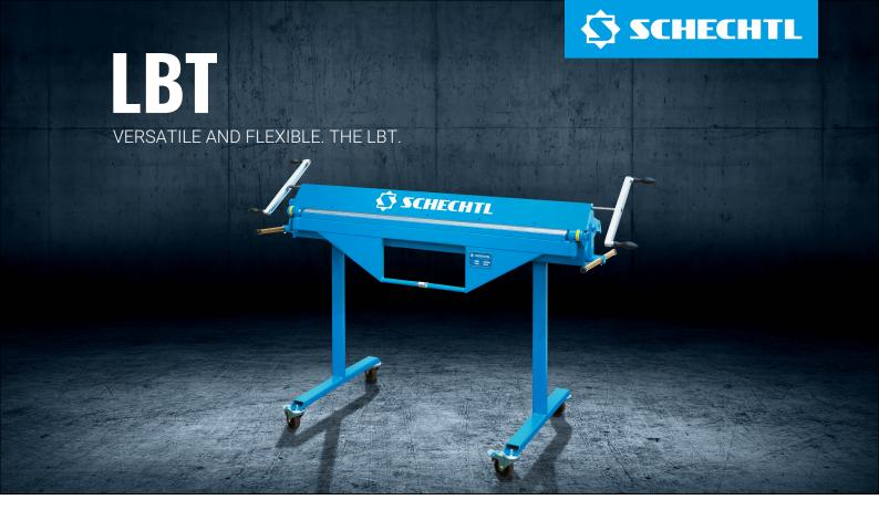
You need a transportable sheet metal bender for cutting, bending and beading? Schechtl has developed one for you! The LBT has a working length of 1290 mm and can bend 1.00 mm steel. The standard equipment includes beading apparatus. The optional roller shear makes the LBT ideal for professional sheet metal forming on the construction site.
