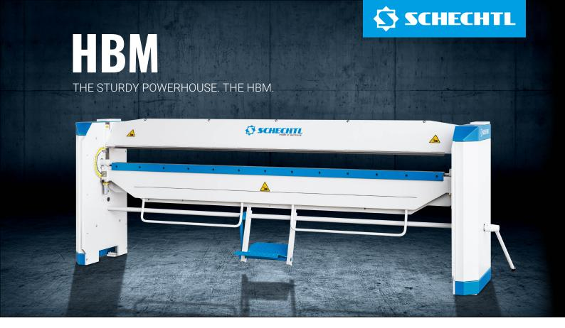
You need a manual sheet metal bender that bends 3-metre sheets? Then the Schechtl HBM is just the right machine for you! The HBM has a bending capacity of 1.00 mm steel, and its design is so robust that it is virtually indestructible. The combination of precision, strength and a wide range of accessories makes the HBM a powerful tool for your workshop.
