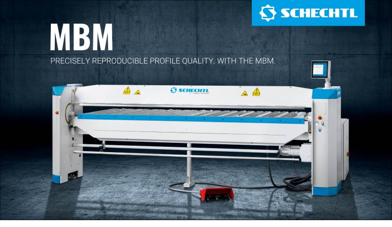
Where manual swivel bending machines reach their limits, the MBM brings you a huge increase in functionality and efficiency. The MBM is ideal for thin-sheet processing of up to 1.00 mm sheet steel, for recurring single-piece production and small batch production Even complex profiles are easily reproducible with the ECT control, which is installed as standard.
